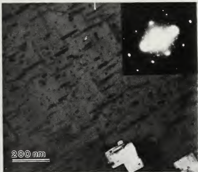
Figure 12B Dark-field TEM Micrograph of 6061 Aluminum Aged for 16 Hours at 473K.
